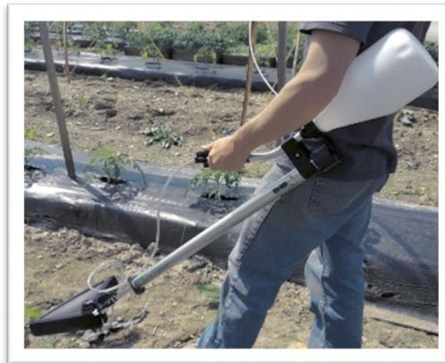
The Herbiflex-4 shown with an A90 head and 2.5 liter bottle can be used with or without a shield. Powered with 4D cell batteries. With low to no drift. Both are great for home owners too.
